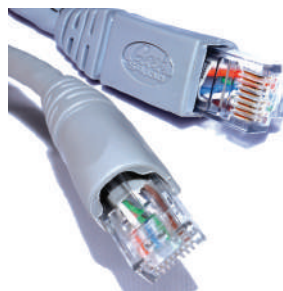
(b):RJ45 UTP connector
