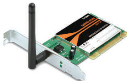
Fig.2.28: Wireless network card
