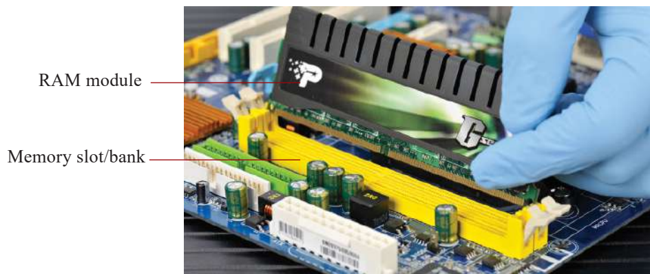
Fig.2.32: Installing RAM modules
