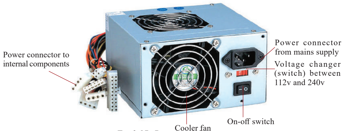
Fig.2.17: Power supply unit.
